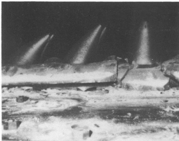
Figure 3 Injector growth after 854 h of ZnSe deposition. The growth cones are around zinc injectors.
